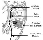
**MST3**: Connect this cable from MST into available terminal on the main body.
