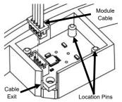
MST2: To position the MST module, ensure the location pins line up and press firmly into Sealing Gromet. Plug the cable provided into the MST module once secured in IPX cover.
