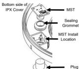
**MST1**: Remove the Plug already in the IPX cover. Replace with the Sealing Grommet.
